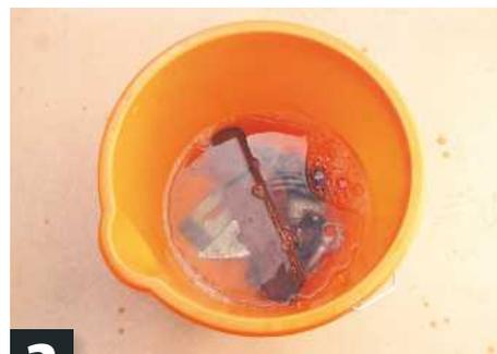
**3** Rinse with hot water, then completely submerge tools in Restore Rust Remover for several hours
